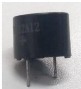
Figura 38: Piezo buzzer
